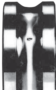
Fig. 5.1 Example of Flaking
